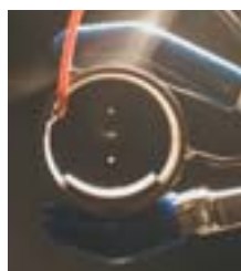
VIBRATIONS trap aerosols along three nodes (white dots).
